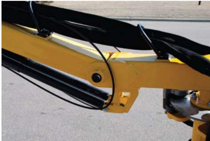
The Spin Doctor ERB-800 works on a primary horizontal axis with a vertical lift in the second arm.
