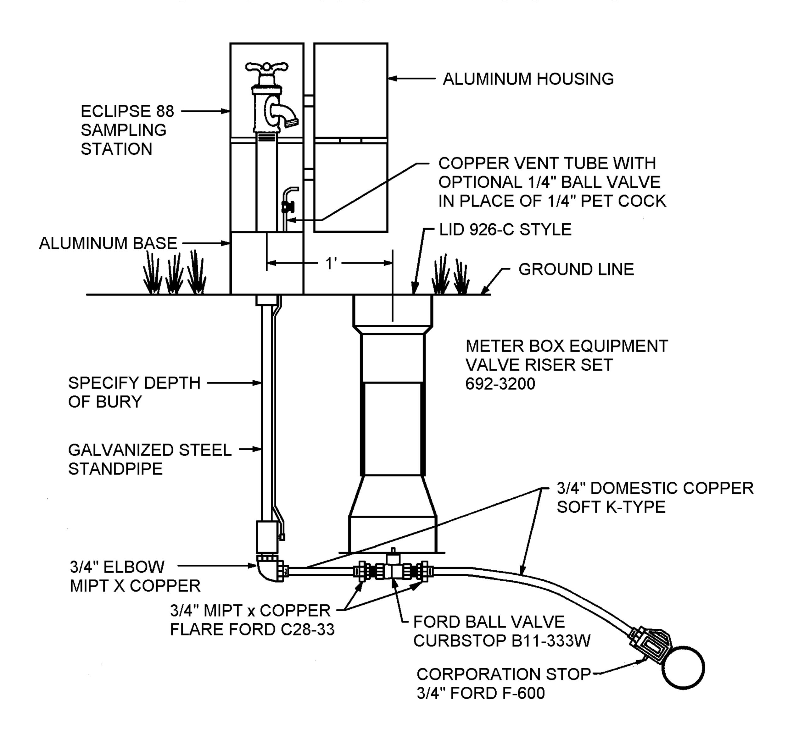
Sampling Stations shall be 'bury, with a 3/4" FIP inlet, and a (3/4" hose or unthreaded) nozzle.
